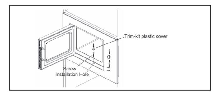
Open the door. Fix the oven to the cabinet with a screw through the installation hole at the front of the trim kit. Once in place, fit the trim kit plastic cover into the installation hole.
