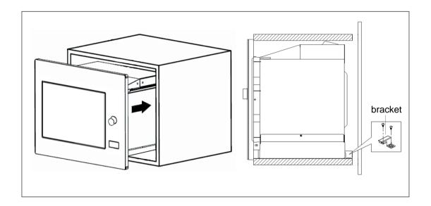
5. Open the door, fix the oven to the cabinet with screw, at the installation hole. Then fix the Trim-kit plastic cover to the installation hole.
