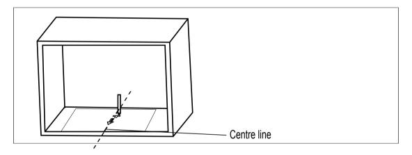
3. Remove the bottom cabinet template and fix the mounting plate with screw.
